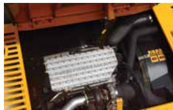
The engine bonnet is compact and opens front-to-rear for easy and safe engine service access.
