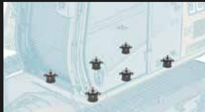
6 nos. viscous mounts to absorb the vibrations that ensures comfort for the operator.
